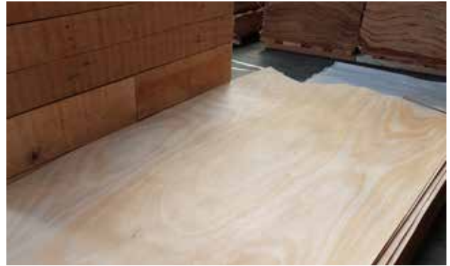
Unrolled veneer sheet © E. Groutel, Wale
