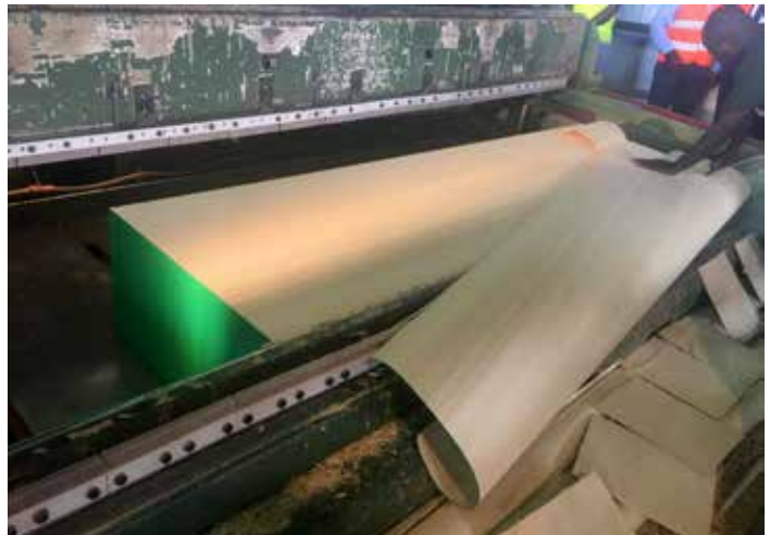
Slicing © B. Jobbé Duval, ATIBT
