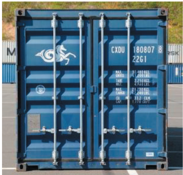
Coding on a container © Emmanuel Groutel - WALE
