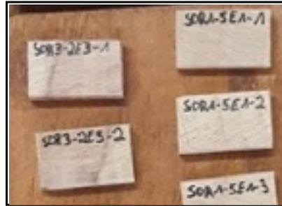
Figure 14: samples for durability tests (fungi and termites)
