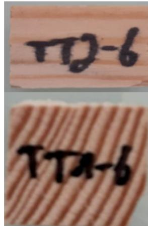
Figure 16: Difference between an L, R, T sample (top picture) and an R, T, L sample (bottom picture)
