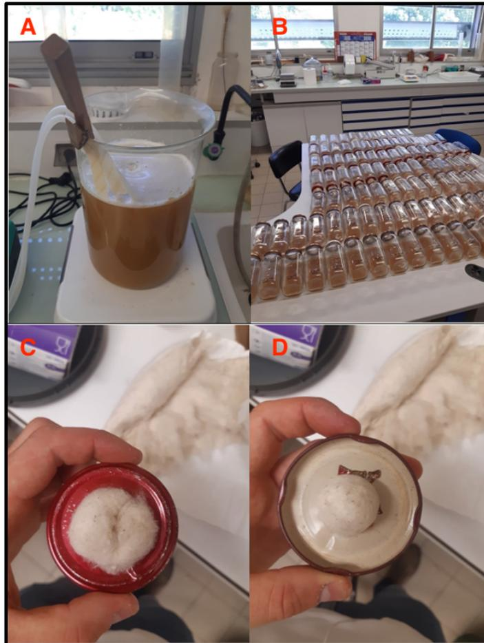
Figure 17: fungal test preparation. A: solution preparation. B: flasks placed. Horizontally to cool down. C, D: cotton caps.
