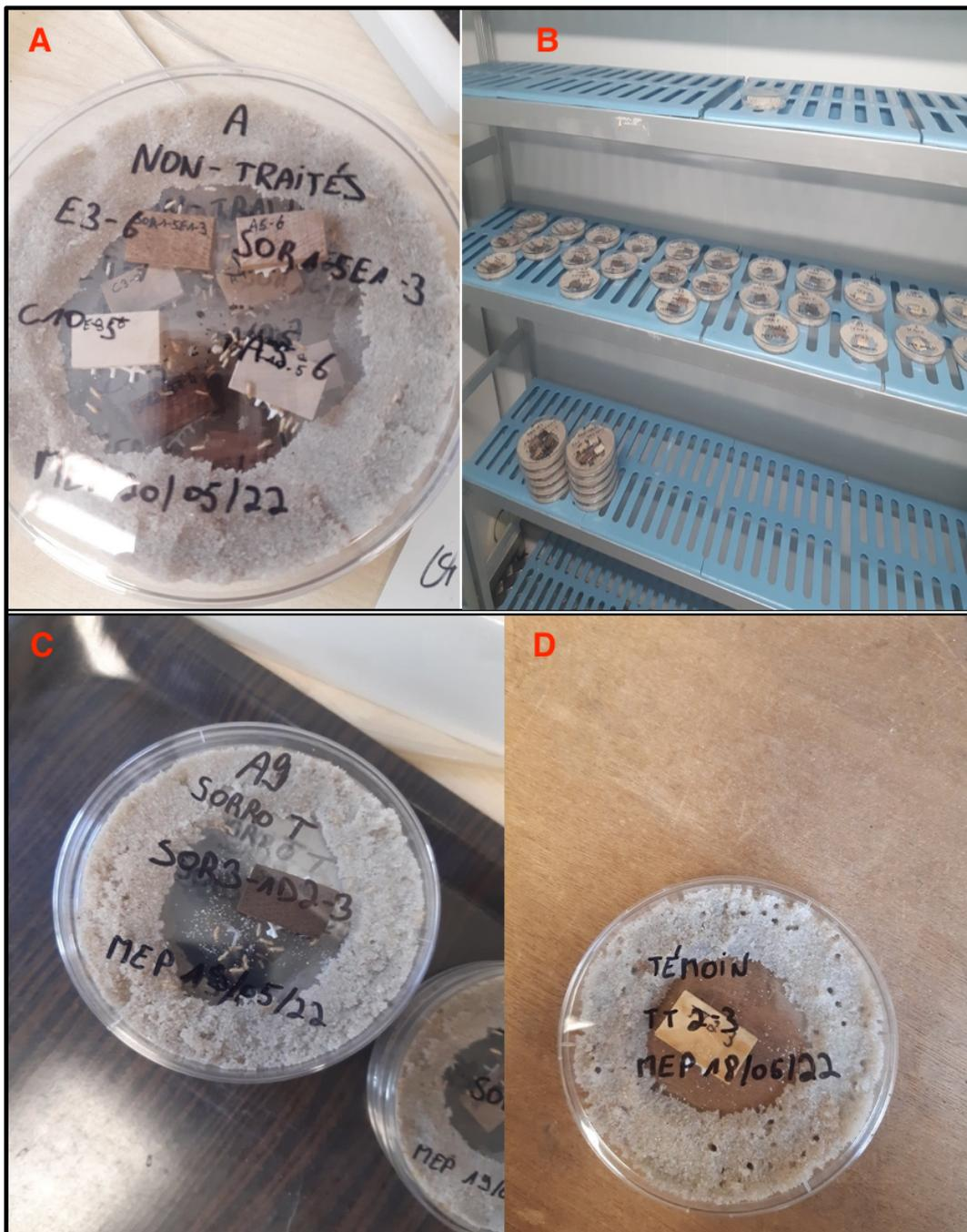
Figure 21: termites tests. A: choice test. B: conditioned room with the Petri dishes. C: nonchoice test with a treated sample. D: Petri dish with a control sample
