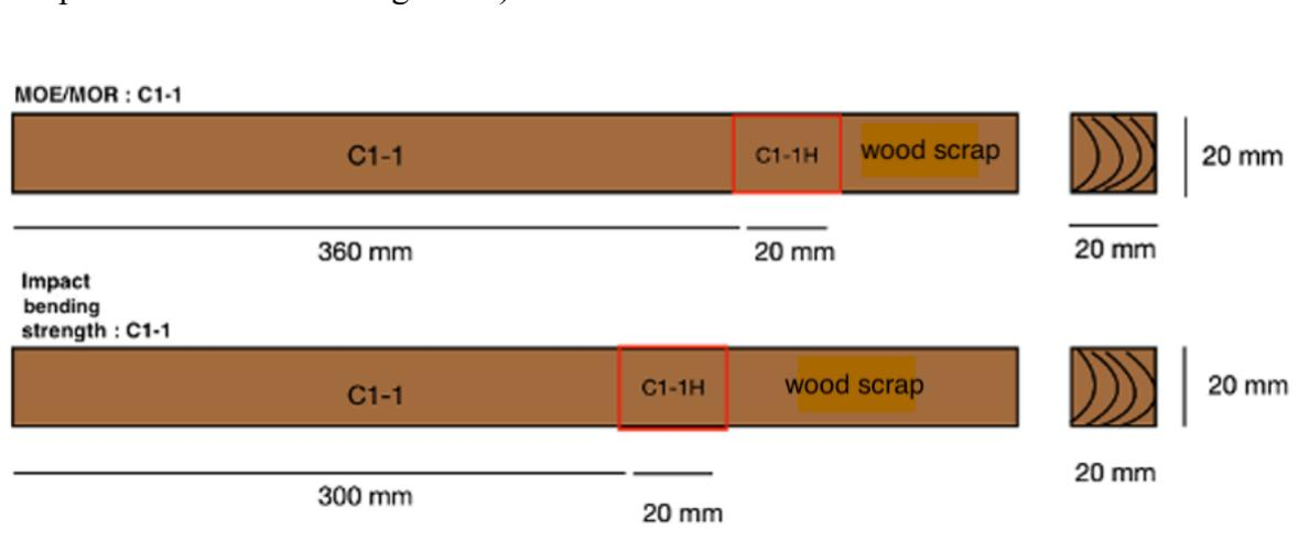
Figure 13: Cutting scheme for MOE/MOR and impact bending strength tests and humidity samples (H)
