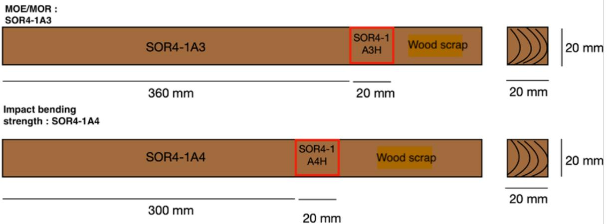
Figure 11: Cutting scheme for MOE/MOR and impact bending strength test and humidity samples (H)
