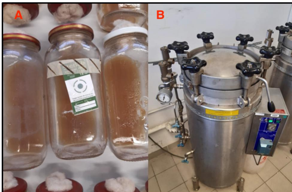
Figure 18: autoclave process. A: control label to prove that the samples have been autoclaved. B: autoclave system
