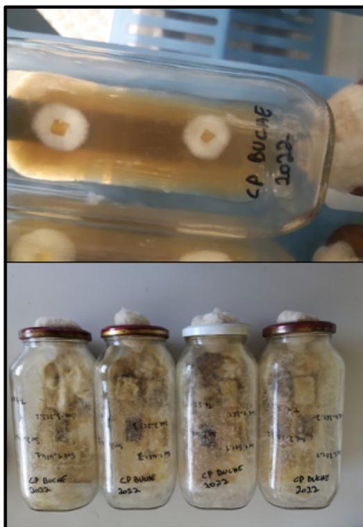
Figure 19: Fungal test. Flask preparation with *Coniophora puteana* (CP). The top picture represents a fungal preparation and the bottom picture shows a fungal test after 8 weeks.
