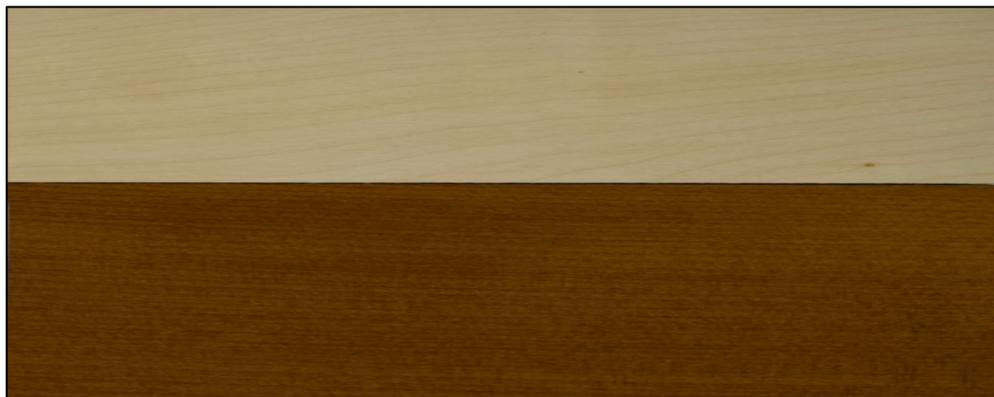
Figure 4 : Color difference between (a) untreated and (b) heat treated *Acer pseudoplatanus*
