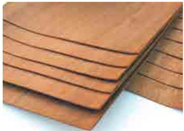
▲ Photo 32: Thick veneering for plywood cores
