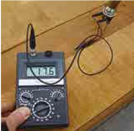
▲ Photo 16: Moisture metre using resistivity
