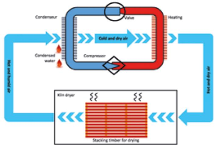
▲ Photo 20: Principle of kiln dryer © P. Martin, ATIBT
