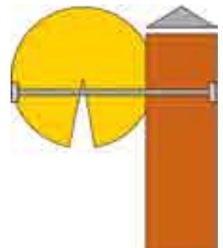
The opening of the cut varies depending on the variations in moisture. It is performed before treatment and it is oriented towards the lower section so that it doesn't create a water trap.
