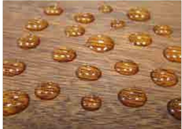
▲ Photo 15: Surface tension of timber © P. Martin, ATIBT
