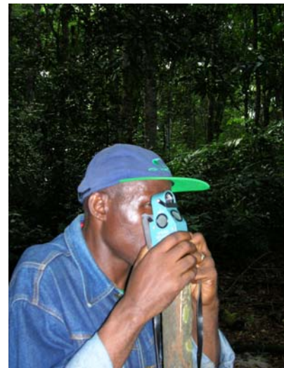
Taking a sighting with the Bitterlich relascope © Benoît DEMARQUEZ
