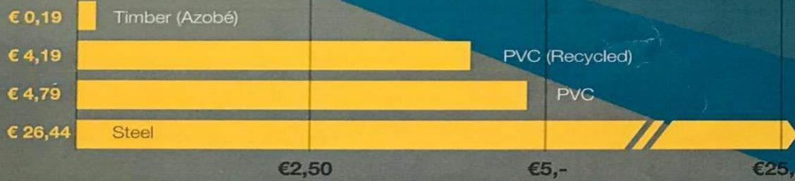
Material ECI per m² of pile planking / sheet piling (EY, 2016)
